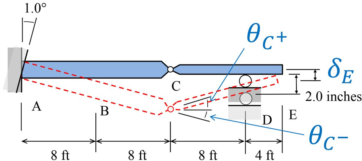
The overhanging beam, from our previous example, has a fixed support at A, a roller support at C and an internal hinge at B.
